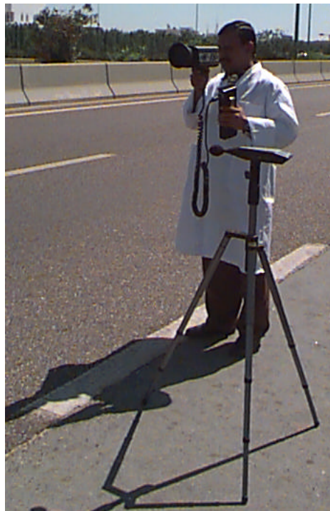
Figure 2.3 Measurement of spot speed using RADAR speed meter
